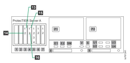
Figure 21. Customer and replication Ethernet connections for single node 10 Gb FSI configuration, Feature Code 3457
