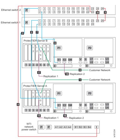
Figure 33. Server B replication ports for OpenStorage configuration, FC 3457
