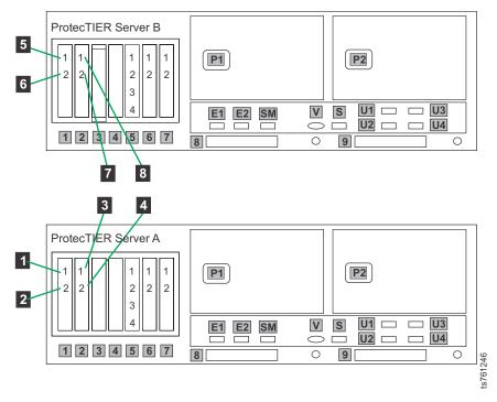
Figure 34. Server B customer host network Ethernet ports for 10 Gb OpenStorage configuration, FC 3457
