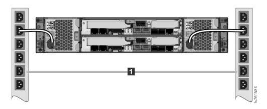
Figure 12. Single node power connections on the DD6
