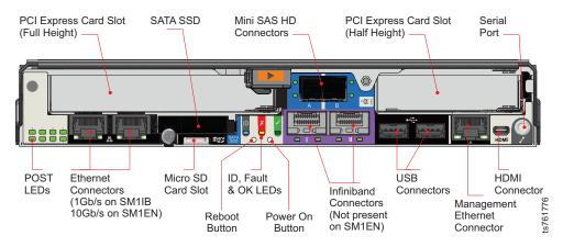
Figure 3. 3958 DD6 server rear view with VTL configuration
