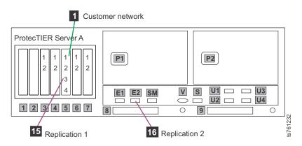
Figure 20. Customer and replication Ethernet connections for single node FSI configuration, Feature Code 3457
