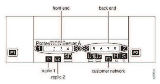
Figure 17. Customer and replication Ethernet connections for single node VTL configuration
