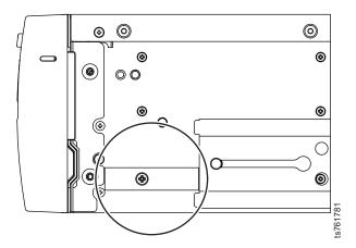
Figure 11. Correct placement of the inner rail stopper
