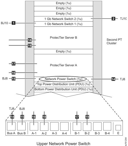
Figure 37. Upper cluster TS7650G power cabling, two clusters in a single frame
