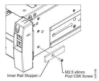
Figure 10. Position the rail stop and screw in place
