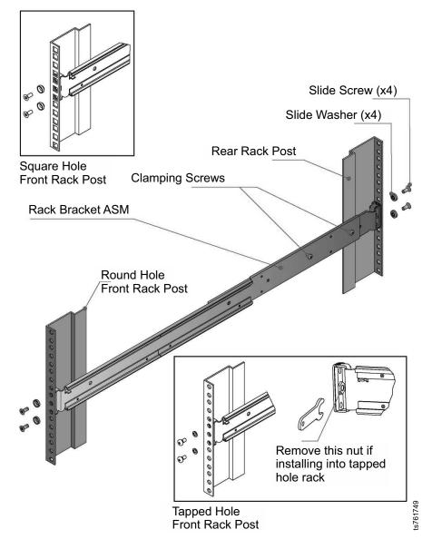
Figure 7. Slide rail components
