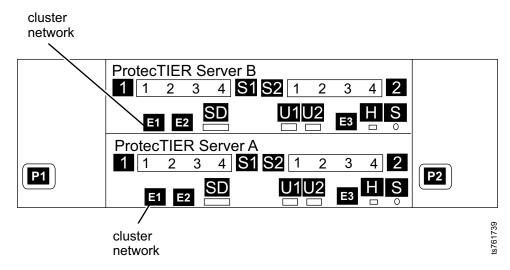
Figure 32. Server B customer host network Ethernet ports for 1 Gb OpenStorage configuration, FC 3456
