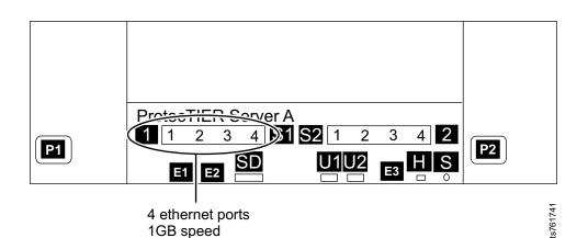
Figure 18. Customer and replication Ethernet connections for single node 1 Gb FSI configuration, Feature Code 3456
