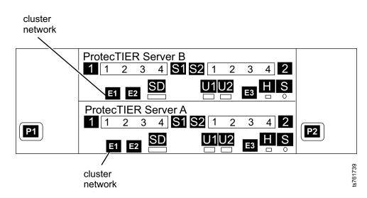
Figure 31. Server B replication ports for OpenStorage configuration, FC 3456
