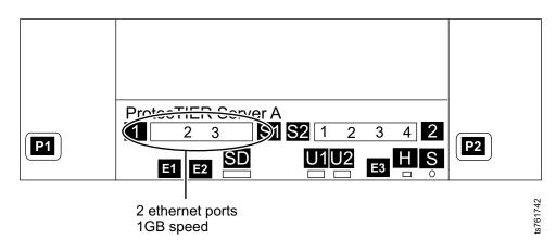
Figure 19. Customer and replication Ethernet connections for single node 1 Gb FSI configuration, Feature Code 3456
