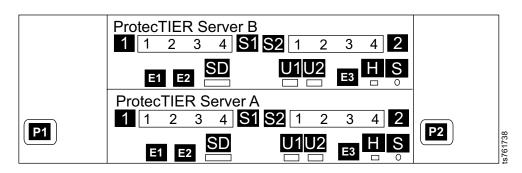
Figure 30. Server B replication ports for VTL configuration
