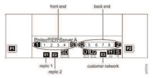
Figure 13. Fibre Channel connections for single node configuration on a DD6
