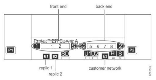
Figure 15. Front-end Ethernet connections for single node configuration on a DD6
