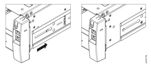
Figure 8. Correct position for the inner rail
