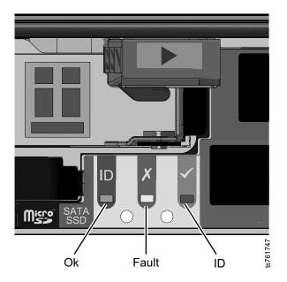
Figure 16. Power on indicators on the rear of the canister
